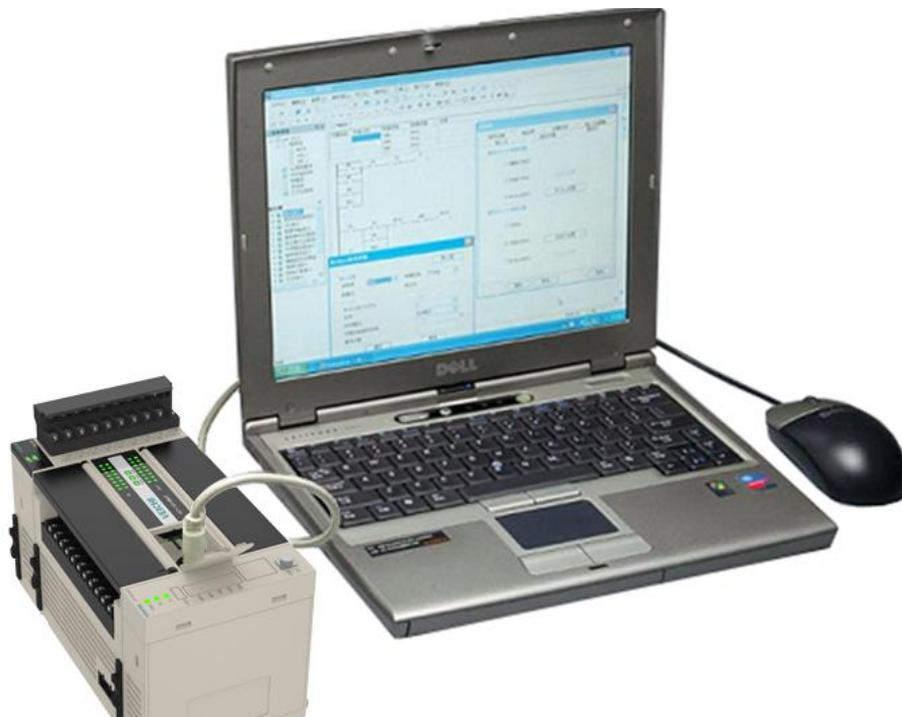
Figure 1-5 Programming cable connection
