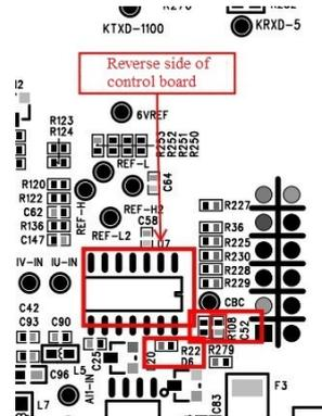
1. Circuit description: In the AC drive wave-by-wave current limiting (CBC) is very
