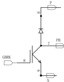
GBRK is the braking signal in the diagram. Connect a braking resistor between terminals P and PB, refer to the instruction manual for specifications.
