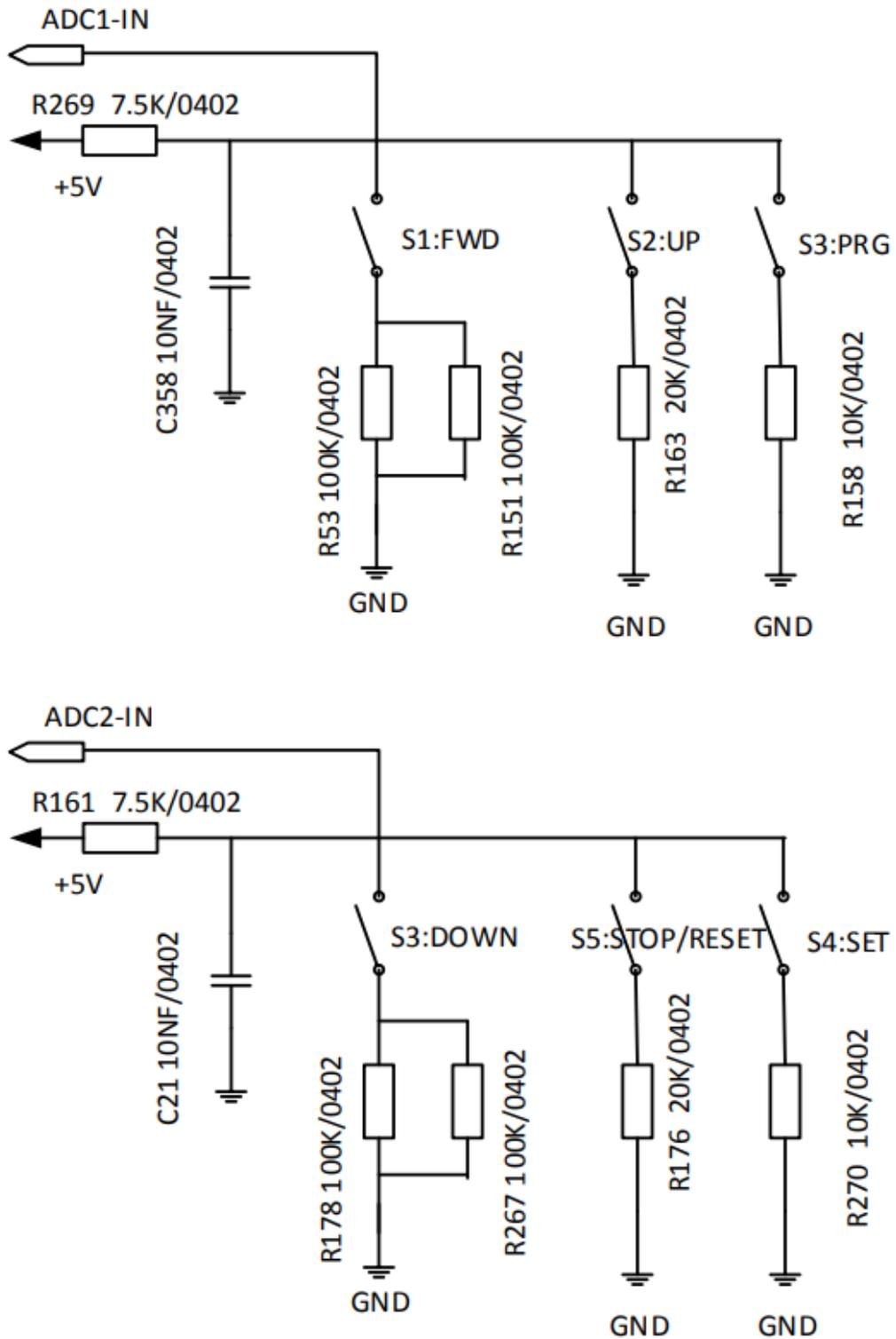
AC300CON1-V1.0 keypad adopts the analogue amplitude detection method to realize the
