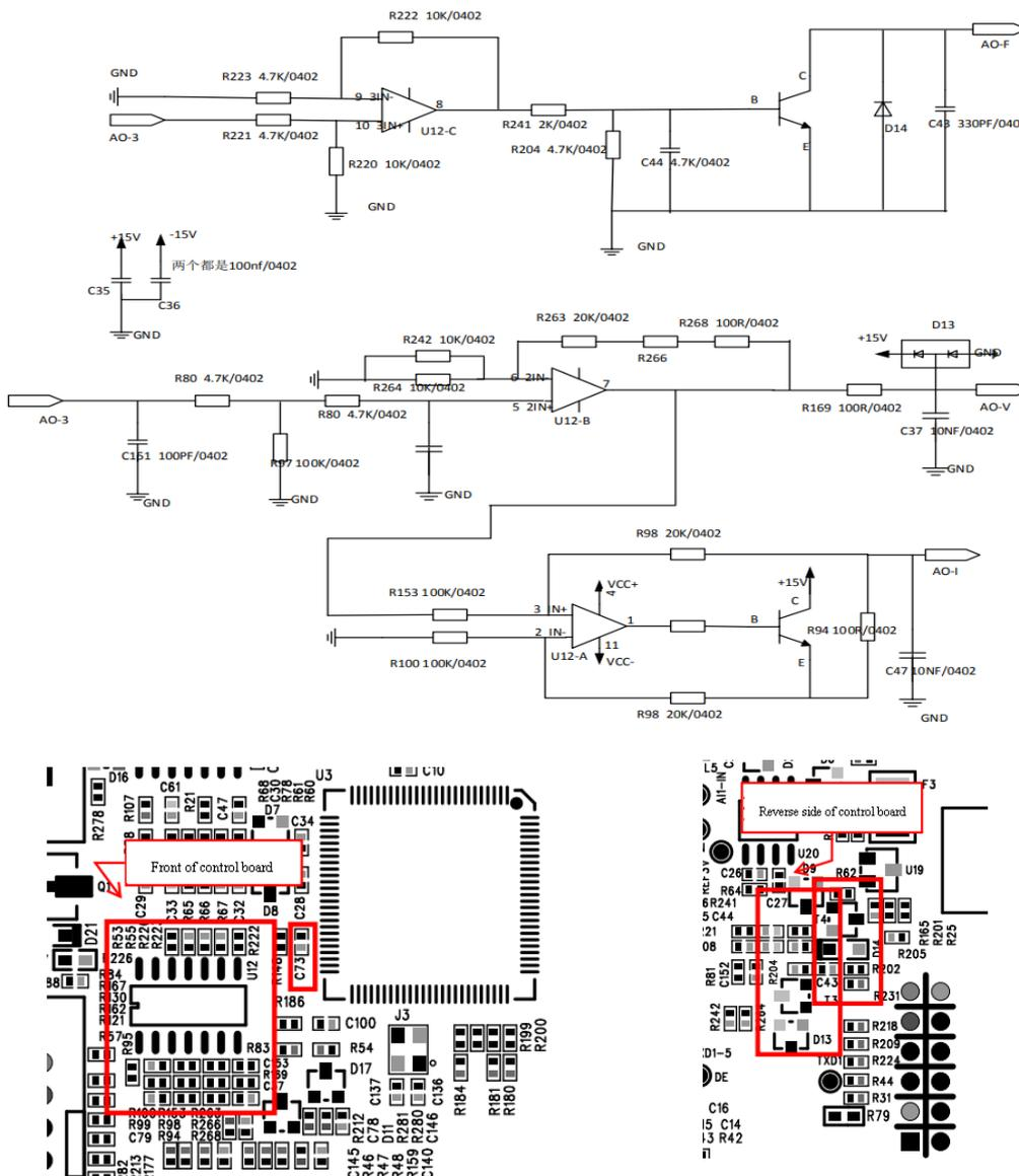
● Test the output voltage: DIP switch to A01 or AO2 voltage ON terminal, at this time parameter setting F03.37=0, F03.38=1, check C00.20 or C00.21, then press the start button, there will be voltage from 0-10V (after parameter setting or use multimeter DC gear, measure +10V).
