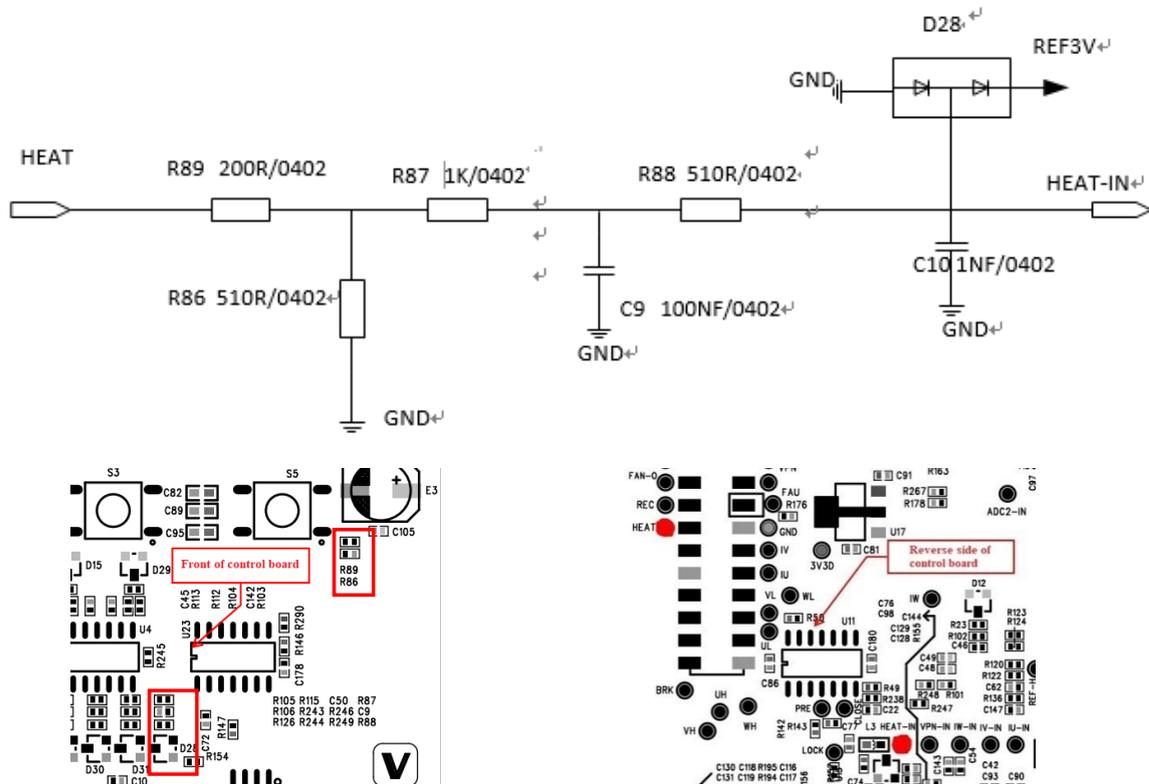
1. GND1 as a reference ground, measuring HEAT, the normal voltage is 0.5V-1V. If the HEAT voltage is abnormal, the power board voltage detection circuit is abnormal, test the power board voltage detection circuit.
