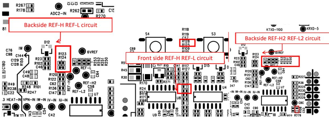
● Output detection at each voltage point: Measure the voltage value of each circuit with a multimeter at DC level.
