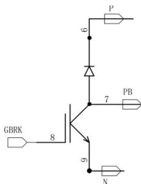
The braking resistor is connected between PB and PJ when the voltage between GBRK and N is about 16 V. Refer to the selection manual for the braking resistor.
