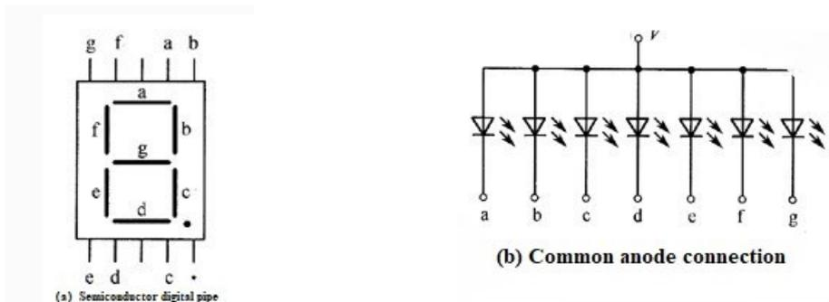
Digital tube repair in accordance with the above digital tube connection diagram and diode repair can be judged good or bad.
