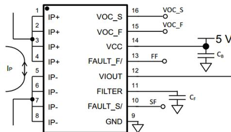
The ACS720 has a user-configurable double-fault function, with fast and slow fault outputs for short-circuit and overcurrent fault detection. Using the fast protection pins VOC\_F and FAULT\_F/, the device sends out a low FAULT signal within 1.5us when the
