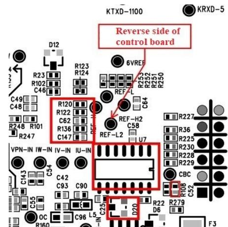
1. Circuit description: in the OC detection circuit, OC threshold for the rated current 2.7 times, in the circuit used in the comparator U7, U8, U9, the comparator provides the reference voltage REF-H, REF-L, the collection of the current IU, IV, IW into the resistor has a voltage, compared with the reference voltage, when between the two benchmarks, will not report a fault, beyond the benchmark will report fault OC.
