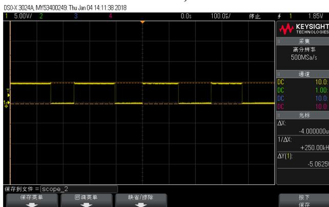
Measured in AC mode during operation, the voltage of each drive signal and GND is about 11.5v.
