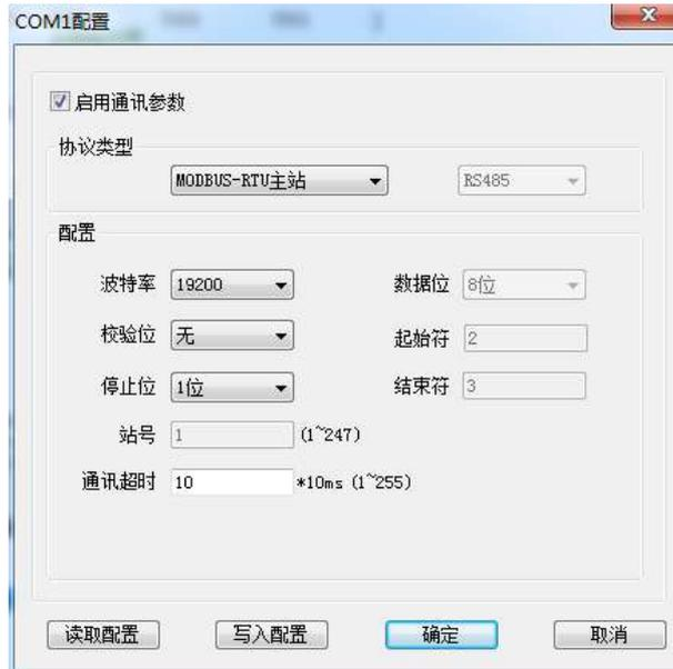
Protocol switching condition: COM1 can switch the protocol when the system is powered on or when the user program is in shutdown state, and the protocol will not be changed in the operation state.
