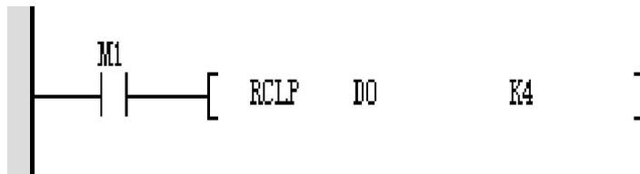
When M1 is on, the number band carry cycle of d0 shifts four bits to the left; The last bit remains in the carry flag bit m8022.
