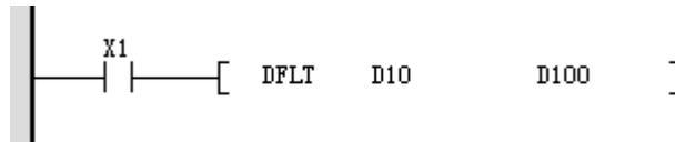
When X1 is ON, the 32-bit number (D11, D10) (32-bit BIN integer) is converted to Binary floating number and stored in (D101, D100).
