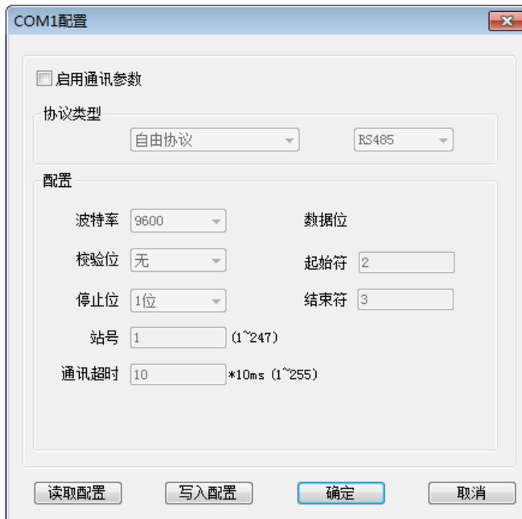
Then select the "enable communication parameters" option, select the "MODBUS-RTU master station" as the protocol type, and modify the required "baud rate", "check bit", "stop bit", "communication timeout" and other parameters. The master station number uses "1" by default, and the modified interface is as shown in the figure below. You can click "read configuration" or "write configuration" to read and set the configuration. Set, click the "OK" button to complete the master station communication
